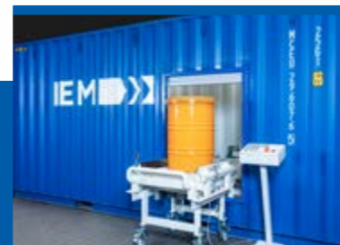
BARREL TIPPING AND TESTING SYSTEM
